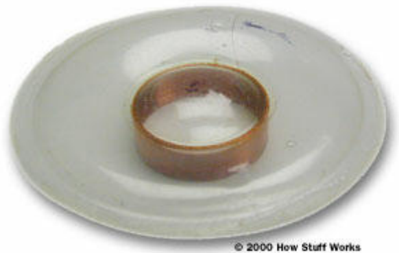
Close-up of the speaker's plastic membrane with attached wire coil
