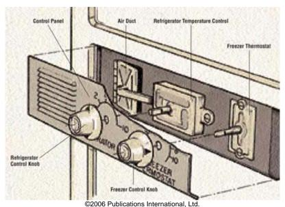
Thermostat controls regulate the temperature of the refrigerator and freezer. Remove the control panel to reach the controls.
