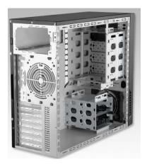
The *computer case* is important because it provides protection for the internal electronic components of the computer. The computer case must also provide sufficient ventilation (so the electronics don't overheat) and room for expansion. Most computer cases are designed to accommodate specific motherboard types.
