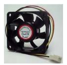
Because computer components generate a lot of heat, the computer *case fan* is essential for maintaining the functionality of the computer. The case fan is the primary source for cooling internal components for most computers (as some custom or higher end computers may use liquid cooling). Some computer cases are built to accommodate additional case fans.
