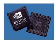
*GPU* stands for *Graphics Processing Unit*. The video card is in charge of controlling the video display. Much like the CPU's relationship with the motherboard, the brain of the video card is the GPU. It is responsible for making the decisions for processing the video card's graphical input and output data. It is often either located under the fan or
