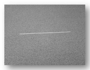
2. Draw a measuring line *perpendicular* to the midpoint of the baseline extending two feet on each side and marked off in half-inches. *Perpendicular* lines are lines that intersect to form a right angle.
