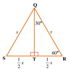
\*Notice that in either of the smaller triangles, the shorter leg is opposite a 30 degree angle and is half of the length of the of one side of the equilateral triangle.
