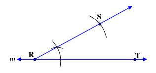
*Step 5*: In this step no further measuring is needed because all of the necessary constructions have been made that satisfy the SAS postulate. In the final step simply draw a segment to connect points S and T to complete the triangle.
