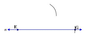
*Step 4*: Move the metal point of the compass to point C of the triangle and adjust the compass so that the pencil point touches point B. The compass will now be set to the length of segment BC. Without changing the setting of the compass, move back to the line and place the metal point of the compass on point G. Make an arc above the line that intersects the other arc. Name the point of intersection, point F.
