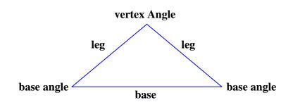
**vertex angle** – The vertex angle of an isosceles triangle is the angle formed by the two congruent sides.
