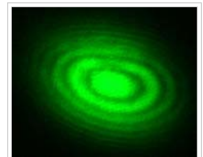
Interference pattern produced with a Michelson interferometer
