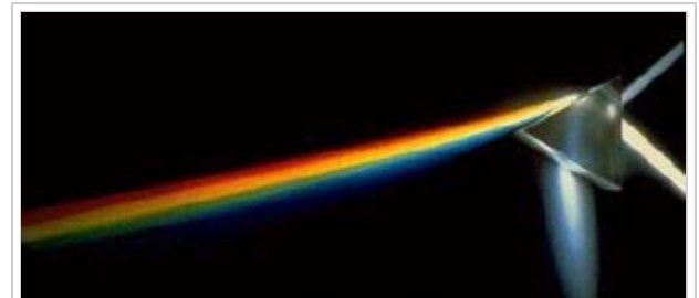
The refractive index of a material indicates how much slower the speed of light is in that medium than in a vacuum. The slower speed
