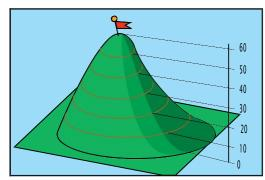
Contour lines show the elevation. Here the land is steeper on the left side and a gentler slope on the right.
