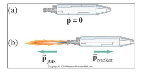
In most linear explosion problems the object will contain two parts after the explosion traveling in opposite directions. It is important to remember then the direction of one of the particles will be negative, therefore giving it a negative velocity.
