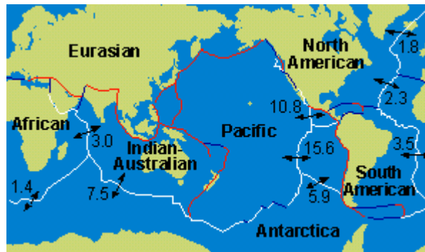
Figure 19. Directions and rates of plate motions (centimeters per year) along oceanic ridge systems. Spreading rates in the Pacific Ocean are nearly five times faster than in the Atlantic. See the global tectonic activity map for more on plate motions.
