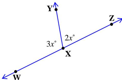
$$\begin{aligned}m\angle WXY + m\angle ZXY &= 180 \\3x + 2x &= 180 \\5x &= 180 \\x &= 36 \\m\angle WXY &= 3x & m\angle ZXY &= 2x \\m\angle WXY &= 3(36) & m\angle ZXY &= 2(36) \\m\angle WXY &= 108^\circ & m\angle ZXY &= 72^\circ\end{aligned}$$
