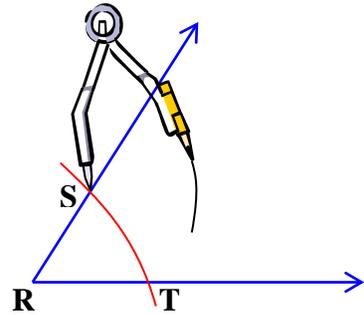
Keep the compass setting the same and place the metal point of the compass at point T. Draw a second arc in the interior of the angle letting it cross the other arc.
