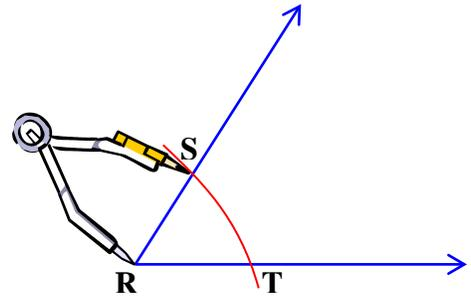
Adjust the compass settings a little wider and place the metal point of the compass at point S. Draw an arc in the interior of the angle.
