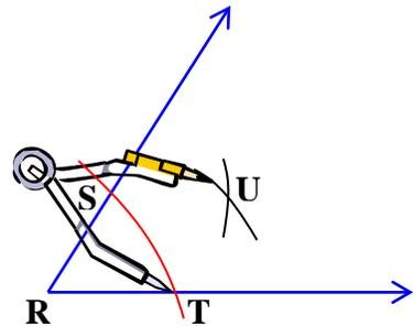
Draw  $\overline{RU}$  so that it starts at the vertex R and extends through the intersection of the two arcs, point U.
